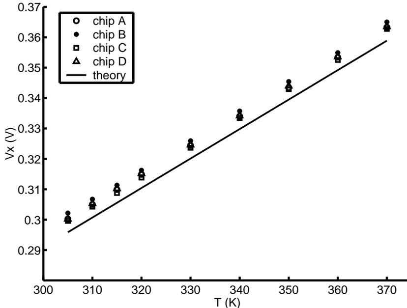
Figure 3: Experimental and theoretical data of the PTAT voltage generator
