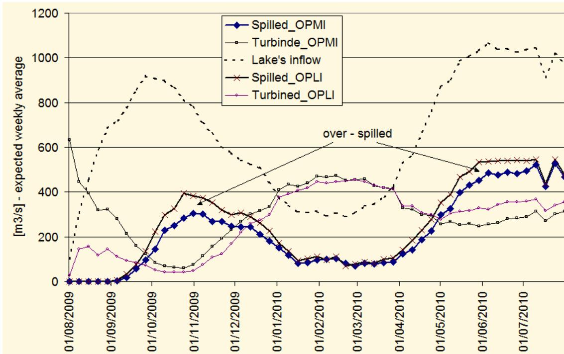
Figure 7. Expected operation of the Bonete hydroelectric plant.
