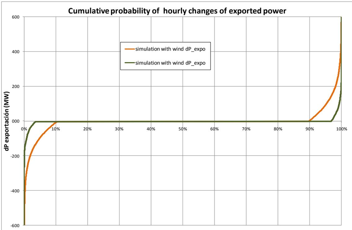
Fig. 6: Cumulative probability of exported power changes from one hour to the next with wind and without wind.
