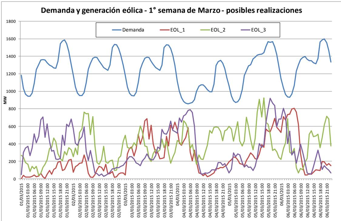
Fig. 2 Simulation of the system demand and wind power generation for a week in 2015
