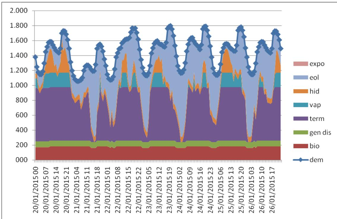
Fig. 8: Hourly simulation of a week with very low hydroelectric generation
