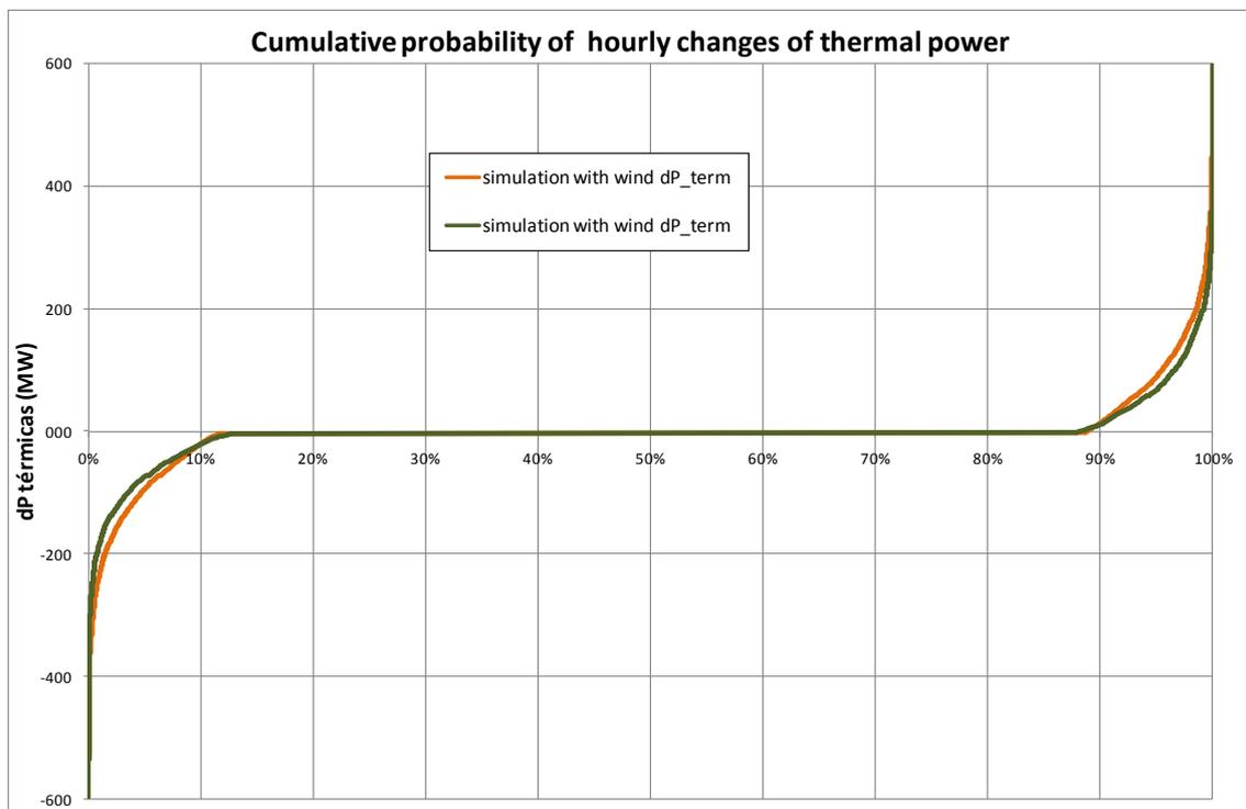
Fig. 4: Cumulative probability of fast thermal power changes from one hour to the next with wind and without wind.
