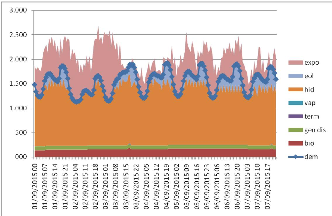
Fig. 7: Hourly simulation of a week with very high hydroelectric generation
