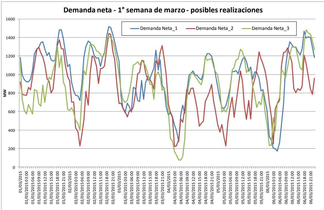
Fig. 3 Net demand to supply (demand- wind power) simulated for a week in 2015
