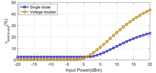
Fig. 18. Simulated conversion efficiency of the rectenna with a rectifier of single diode and voltage doubler.
