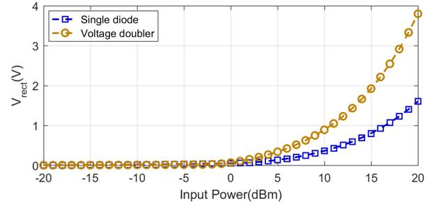
Fig. 17. Simulated rectification voltage of the rectenna with a rectifier of single diode and voltage doubler.
