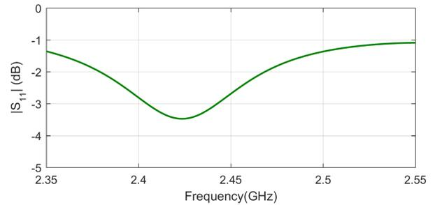
Fig. 9. Simulated  $S_{11}$  magnitude of tuned antenna with calculated filter.
