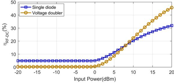
Fig. 15. Simulated conversion efficiency of the single diode rectifier and the voltage doubler.
