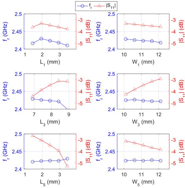
Fig. 10. Characterization of resonant frequency (left axis) and  $S_{11}$  magnitude (right axis) of the filter with antenna.
