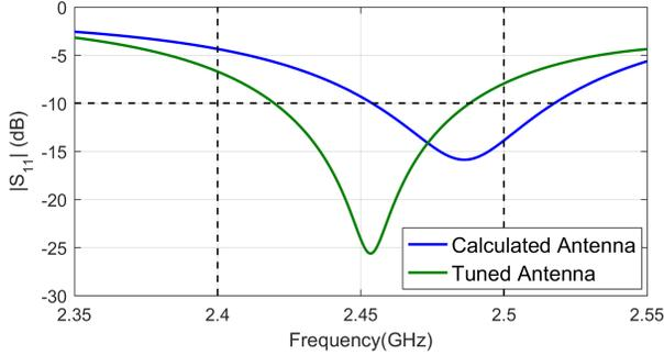
Fig. 5. Simulated  $S_{11}$  magnitude of calculated and tuned antenna.
