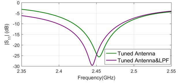
Fig. 12. Simulated  $S_{11}$  magnitude of the tuned antenna and the combination of the tuned antenna and filter.
