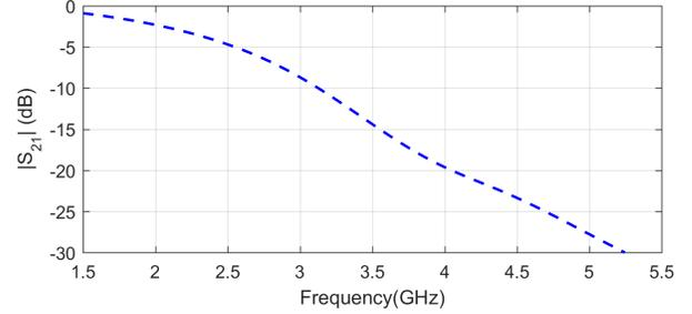
Fig. 8. Simulated  $S_{21}$  magnitude of calculated LPF.
