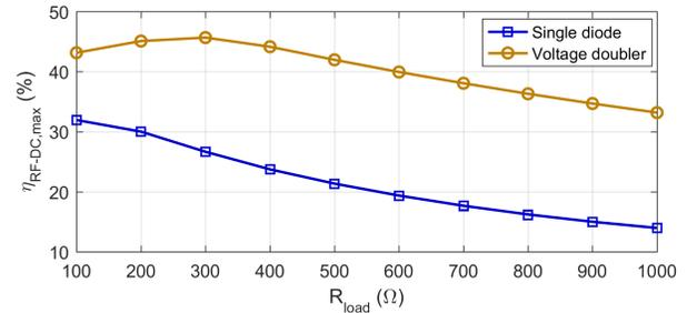
Fig. 14. Simulated conversion efficiency of the rectifiers as function of the load impedance.
