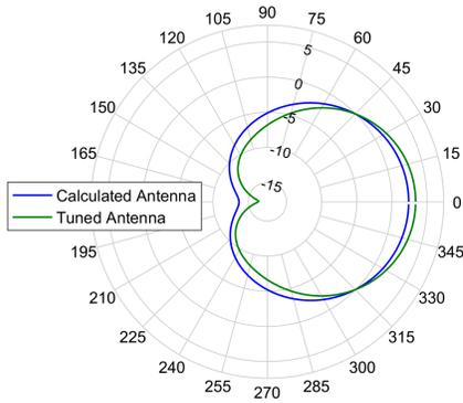
Fig. 6. Simulated gain in H plane of calculated and tuned antenna.
