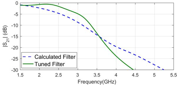
Fig. 11. Simulated  $S_{21}$  magnitude of calculated and tuned LPF.
