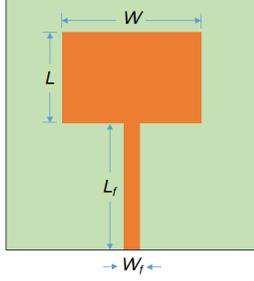
Fig. 2. Dimensions of the antenna.
