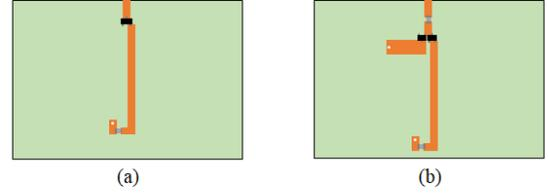
Fig. 13. Rectifier circuit with single diode (a) and voltage doubler (b).
